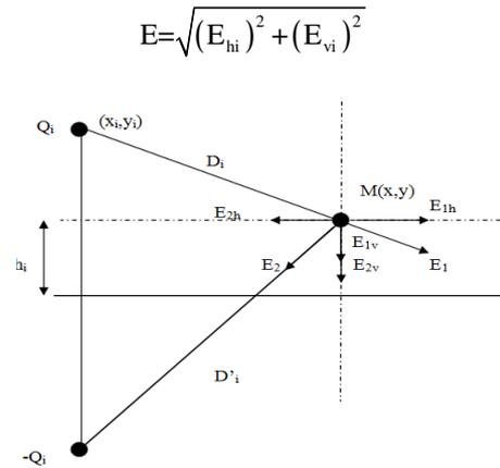
Fig.3: Components of electric field due to HVPL
