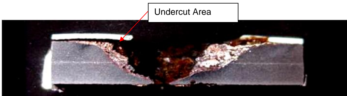
Figure 7. Metallographic Cross Section – Stray D-C Interference Corrosion (4-inch FBE Coated CS Pipeline)
